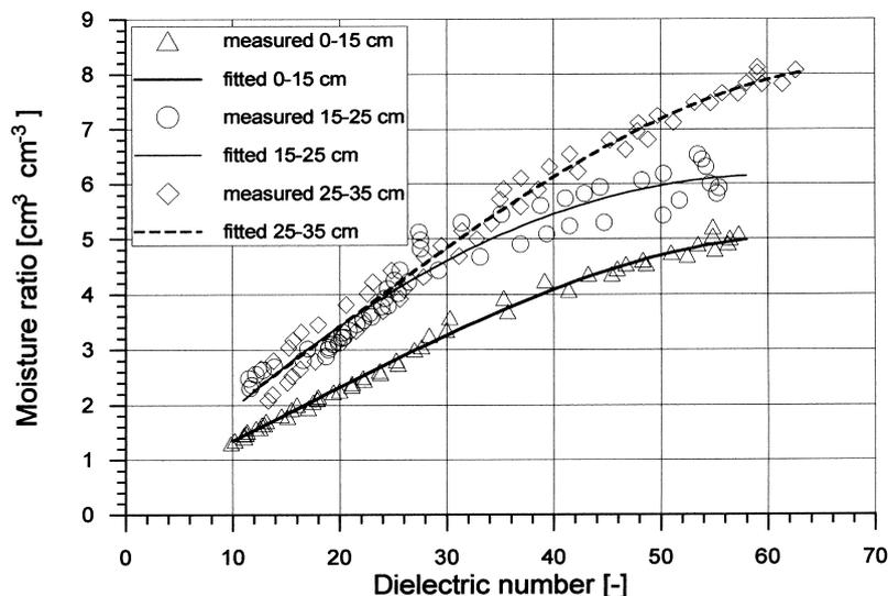
Fig. 2. TDR calibration curves for different peat-moorsh soil layers.
