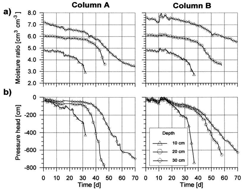
Fig. 3. Moisture ratio (a) and pressure head (b) changes during the drying of peat-moorsh soil columns.
