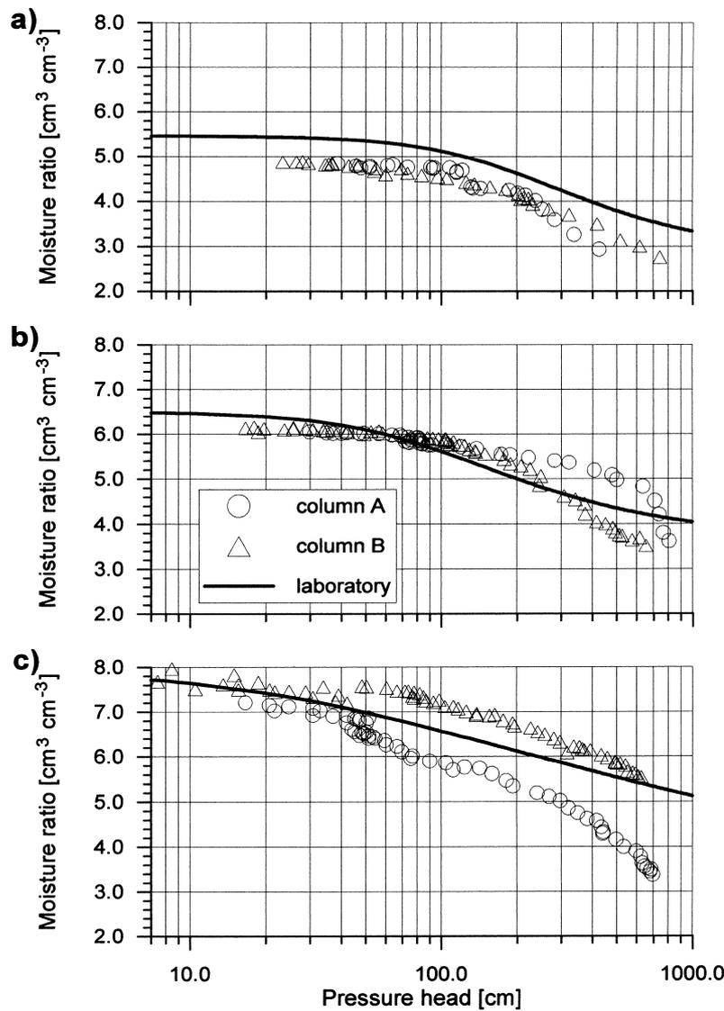
Fig. 4. Comparison of laboratory and field measured soil moisture characteristics for the following soil layers: a) 0–15 cm, b) 15–25 cm, c) 25–35 cm.
