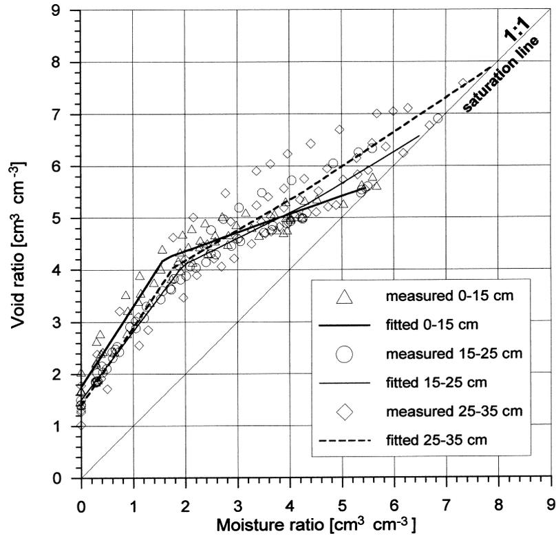
Fig. 5. Measured and fitted shrinkage characteristic curves for different soil layers.
