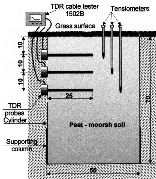
Fig. 1. Scheme of the soil column.
