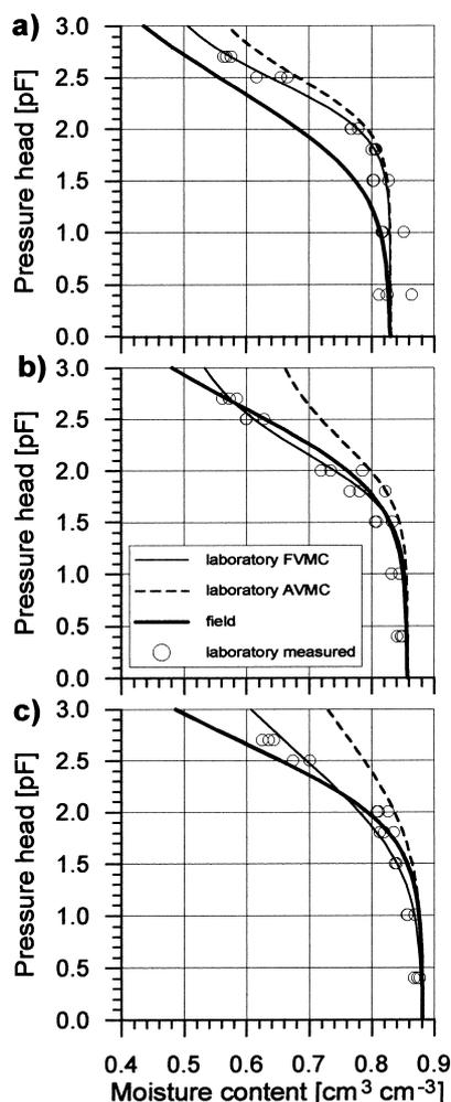
Fig. 6. Comparison of soil moisture retention characteristics measured in the laboratory as related to fictitious (FVMC) and actual volumetric moisture content (AVMC) with field measurements for the following soil layers: a) 0–15 cm, b) 15–25 cm, c) 25–35 cm.
